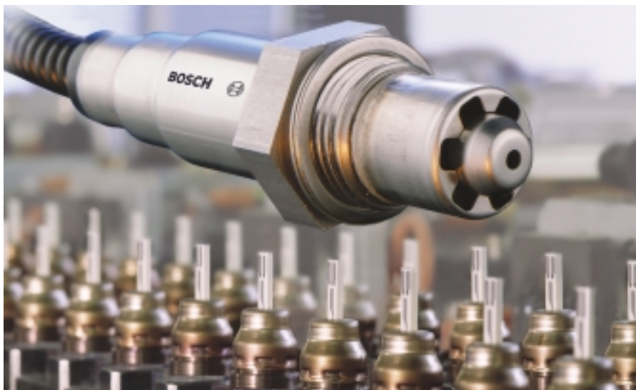
Lambda or oxygen sensors, which contain platinum electrodes, are essential components of auto emissions control systems. By continuously monitoring the engine exhaust composition they enable catalytic converter efficiency to be maximised.
