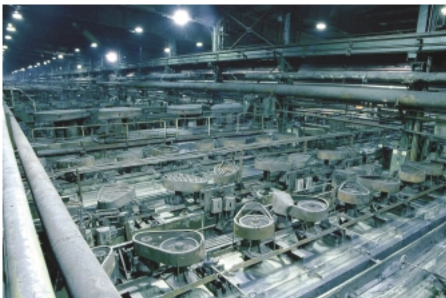
Banks of flotation cells at Norilsk Nickel's Taimakh operation on the Taimyr Peninsula in Siberia.
